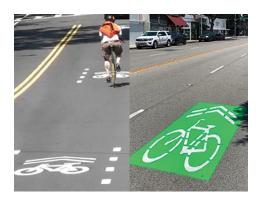
An on-street bike lane is space in the roadway designated for bikes only with striping or pavement markings.
